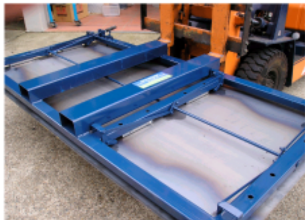
Mag-Frame in use with Forklift
