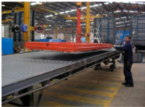
One of four automated Mag-Frames used by MaxiTrans to lift and transport checker-plate sheet
